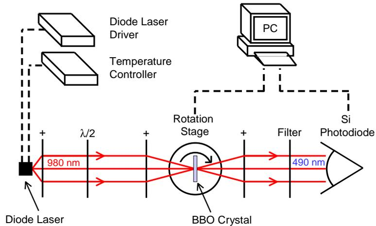
Figure 1: *Experimental setup used for the second-harmonic generation. An incident beam from a diode laser at a wavelength of 980 nm is focused into a crystal of BBO. Here a small fraction of the incident light is converted into light at the double frequency leading to a faint blue beam at a wavelength of 490 nm. The 490 nm light is filtered out and its intensity can be measured using a sensitive photodiode.*
