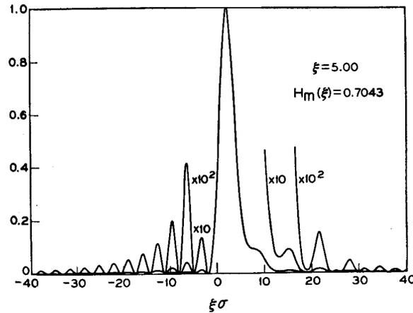
Figure 8: Second-harmonic intensity as a function of the tilt angle of the birefringent crystal, expressed in terms of the phase mismatch  $\frac{1}{2}\Delta kL = \xi\sigma$  for a relatively thick crystal  $\xi = 5.0$ .
