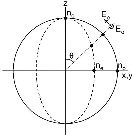
Figure 3: Plot (exaggerated!) of the ordinary and extra-ordinary refractive index at a single wavelength for different propagation directions. A line from the origin corresponds to propagation at an angle  $\theta$  relative to the c-axis. The two intersections yield the ordinary and extra-ordinary refractive index. The direction of the E-field for ordinary and extra-ordinary polarization is sketched in the figure as well.
