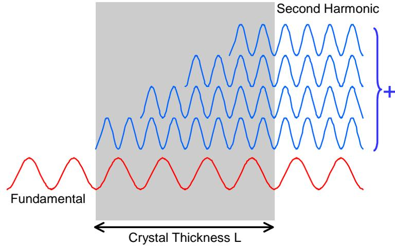
Figure 2: A sketch of the concept of phase matching. The fundamental wave at frequency  $\omega$  has a well defined phase and amplitude everywhere in the crystal. The induced dipoles all radiate at a frequency  $2\omega$  with a phase dictated by the fundamental wave. The picture shows the case where all dipoles radiate in phase in the forward direction so that all contributions add up constructively.
