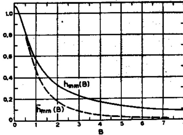
Figure 7: Second-harmonic intensity, expressed in a scaled function  $h(B, \xi)$ , versus the walk-off parameter  $B$ . The solid curve corresponds to the process of second harmonic generation (see text).
