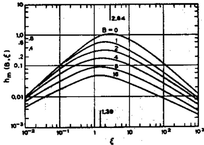
Figure 6: Second-harmonic intensity, expressed in a scaled function  $h(B, \xi)$ , versus the focusing parameter  $\xi = L/b$  for various walk-off conditions  $B$  (see text).
