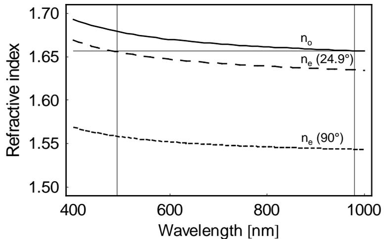
Figure 4: Refractive index as a function of optical wavelength for BBO. The lines in the figure correspond to the ordinary and extra-ordinary refractive index. Also indicated is the index calculated for  $\theta = 24.9^\circ$  that yields perfect phase matching for frequency doubling of 980 nm light.
