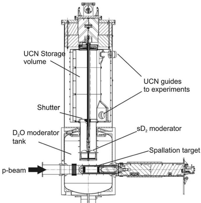
**Fig. 2.** Layout of the UCN source at PSI. The proton beam hits the spallation target from the left. Spallation neutrons will be thermalized in the ambient temperature  $\text{D}_2\text{O}$  moderator, further cooled and downscattered into the UCN regime in the cold  $\text{sD}_2$  moderator. The UCN reaches the storage volume via a vertical neutron guide where they can be trapped and distributed to the experiments.
