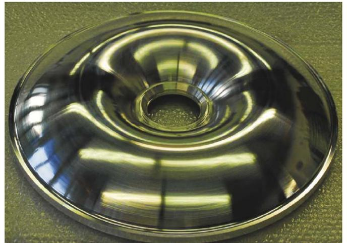
**Fig. 3.** The toroidal lid for the  $\text{sD}_2$  converter made from  $\text{AlMg}_3$ .
