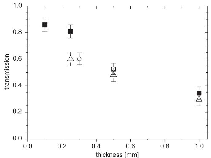
Fig. 4. Transmission of slow neutrons with velocities  $5 \text{ m/s} \leq v \leq 9 \text{ m/s}$  through material foils.  $\text{AlMg}_3$  (black squares),  $\text{Zr}_{110}$  (open triangles) and  $\text{Zr}_{125}$  (open circles).
